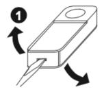
Remove the portable receiver battery cover and remove both AA batteries
