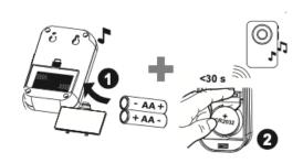
Place both of the AA batteries back into the portable receiver (ensure correct polarity is observed) and within 30 seconds push the small white button mounted internally on the mat transmitter circuit board. The receiver should now chime to indicate it has been unpaired from the mat transmitter. Now replace the battery cover on the mat transmitter. (At this point you should repeat steps 1 and 2 on any other mat and receiver combinations you wish to work separately).
