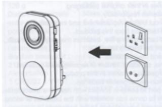
Remove the Mains Powered receiver from the wall socket
