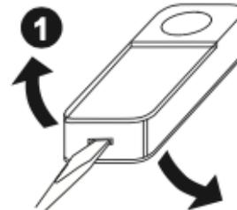
Now remove the battery cover on the mat transmitter by inserting a small flat bladed screwdriver into the slot on the end of the transmitter
