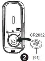
Now remove the battery cover on the mat transmitter unit by inserting a small flat bladed screwdriver into the slot on the end of the transmitter. Insert the coin battery into the mat mounted transmitter unit, positive (+) side facing up, and replace the transmitter battery cover.
